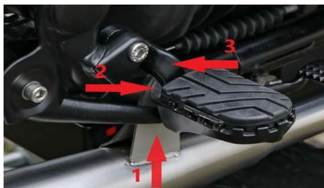
1 – Silencer bracket, 2 – Aluminium spacer sleeve, 3 – Footrest panel (Shown version for right hand side, left hand side has to be mounted accordingly)
